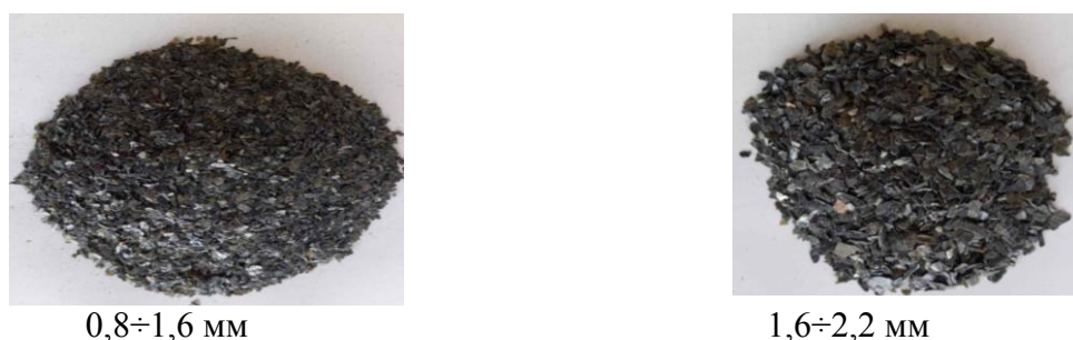
Figure 1. Grinding from Tebinbulok vermiculite mine ore and to different grain sizes obtained by beneficiation silver and gold vermiculite concentrates
