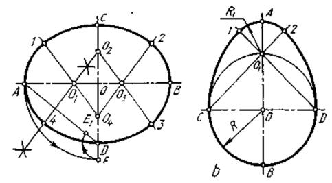
An ovoid is a curve with an ovoid contour, and it is convenient to draw it through the minor axis SO. A circle with a diameter of SO is drawn, and its intersection with the major axis AV is marked as O<sup> $^$ </sup>. S and O<sup> $^$ </sup>, O and O<sup> $^$ </sup> are connected and continued. From point O, 12 arcs with radius OS are drawn from point S1,0<sup> $^</sup>$ </sup> with radius O<sup> $^$ </sup> V, and 2O arcs with radius SO are drawn from point S.
