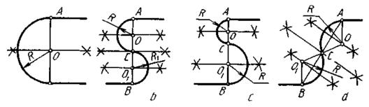
The point of intersection of two circles lies on the line connecting their centers. If two circles touch each other with their outer sides, it is called an external connection, and if the smaller circle touches the inside of the larger circle, it is called an internal connection. In the external connection, the center of the circle is equal to  $K+K^{\wedge}$ , and in the internal connection, their distance is equal to K-K.-].
