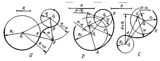
Connecting one of the circles with external and internal compound connection at the given radius is  $K.>0^{0} 02 + K^{K}2 / 2$  only if 0-| from K-K^, 0? arcs with radii K+K2 are drawn from and intersected. During 00^, the transition points V between A, 002 are found and the connection with radius K from 0 is performed.
