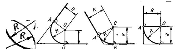
If two straight lines are parallel to each other, an auxiliary line perpendicular to both is drawn to round them. A and B are bisected is divided, the rounding center is 0. Here, one return has a rounding radius. If it is necessary to round parallel straight lines in two radii, then the rounding
