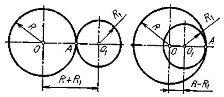
Circles with centers  $O^{\wedge}$ ,  $0^{\wedge}$  are formed by crossing the outer side of the third circle with center 0. To find the center 0 in the outer joint, an arc with a radius of K+K^ from 0, and an arc with a radius of K+V.2 from 02 are drawn and intersected. In determining the center 0 in the internal connection, the arcs drawn from O^ to K.-K.^ ,0^ to K-K^ RaDiUs are intersected.
