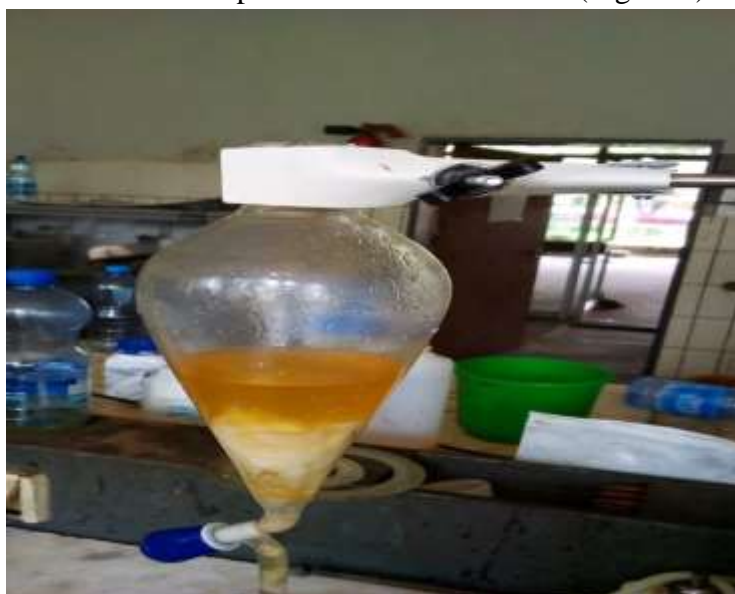
Figure 4: crude oil washing and neutralization
