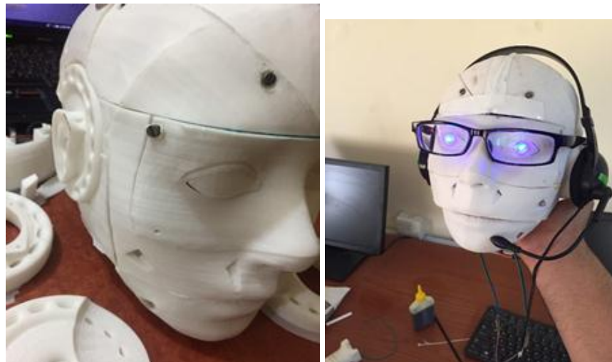
Fig. 3: Head of the ASH robot (3D printing).
