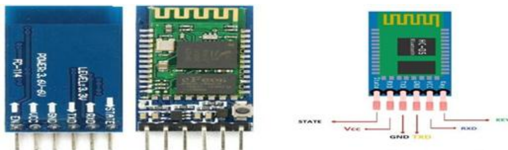
Figure 2.2. Bluetooth module HC-05 configuration.
