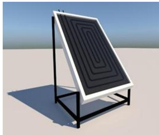
The experimental results indicator on the device of the solar water heat collector with high thermal efficiency, which has low hydraulic resistance due to solar water heaters with different geometric shapes, is presented below. The length of the tubes in which the supplied collector was located was about  $l = 18\text{m}$  in length when placed by calculation, while the length of the Collector surface by  $h = 1,4\text{m}$  by width by  $a = 0,7\text{m}$  gave the Surface  $S = 1\text{m}^2$ .
