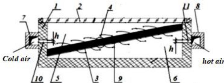
**Picture.** Solar air heating collector with absorber made of metal wire mesh.
