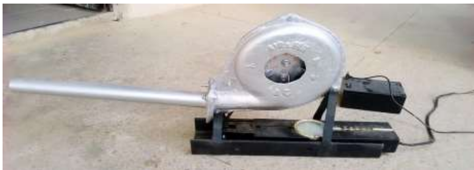
Figure 3. Construction of a Solar-Powered Blower
