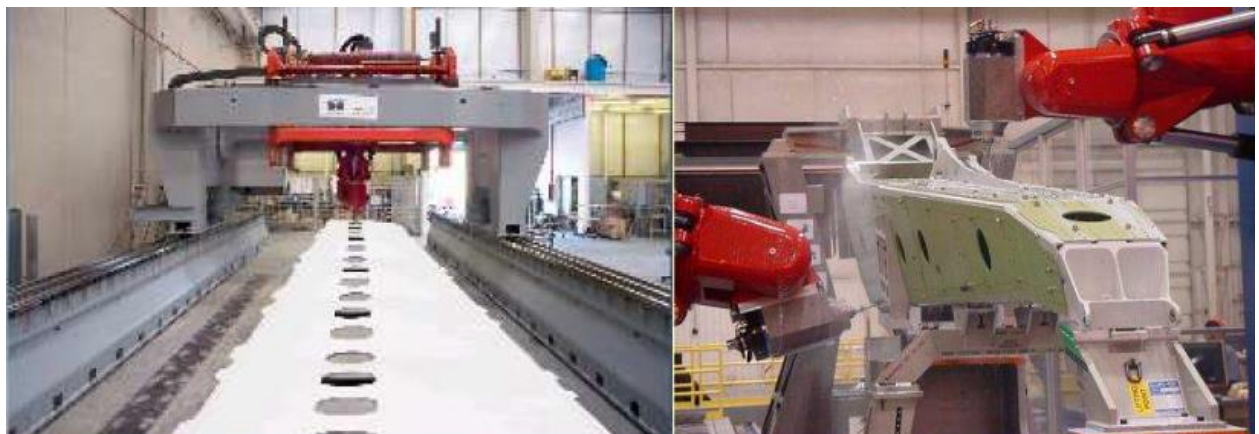
Figure 6. Examples of using a machine with hybrid kinematics for processing large parts
