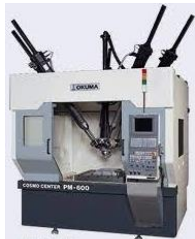
Figure 5. Machine with parallel kinematic structure using OKUMA PM-600V variable length rods
